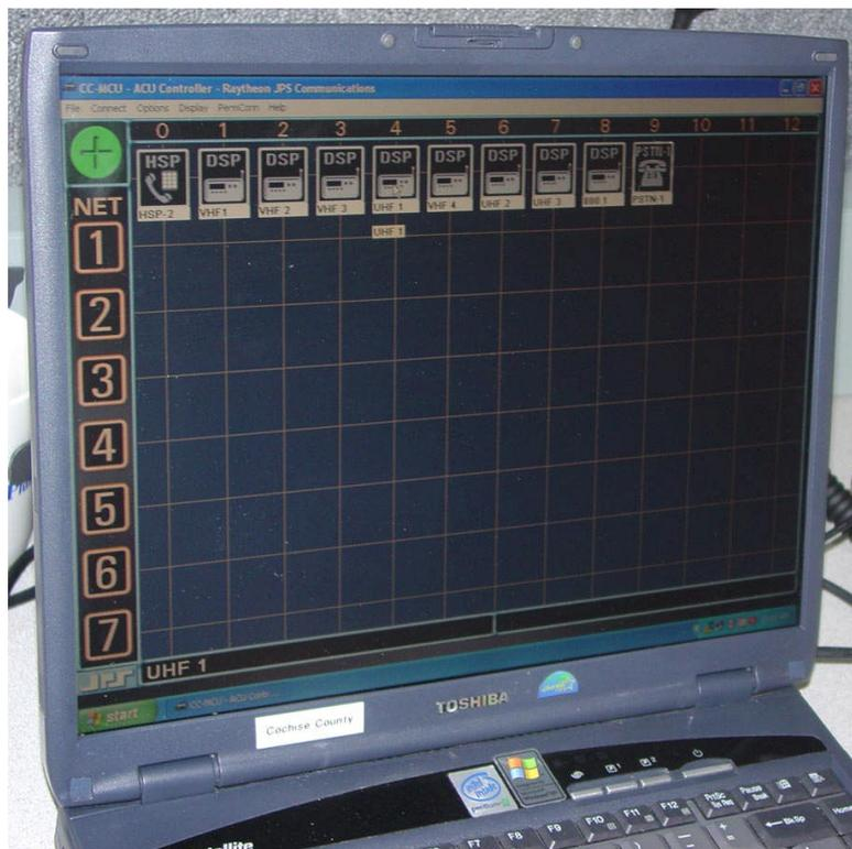
Above each icon is the module's slot number (00-12), referred to as the Module Number. An empty slot is represented by a blank space where the module's icon would appear. Each icon bears the module type name at the top (e.g. DSP-1). When modules are connected (linked), their icons drop to a net line. All icons placed on a given net line
