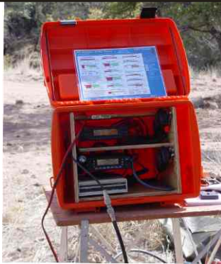
VHF/UHF Station Operating in box Starting to rain
