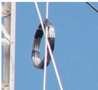
Balun: 7 turns of coax tightly wrapped and taped. Directly below matching section.
